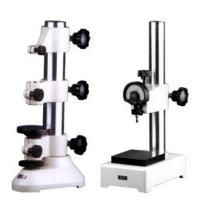
Comparator Stands are basic building-blocks for the assembly of special-purpose, precisionmeasuring equipment. By mounting precision-measuring instruments onto the stands, all types of measurement including comparative measurement is possible.
